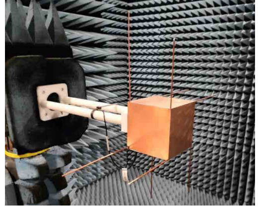
Fig. 1. VHF antenna integrated in a CubeSat structure [5].
